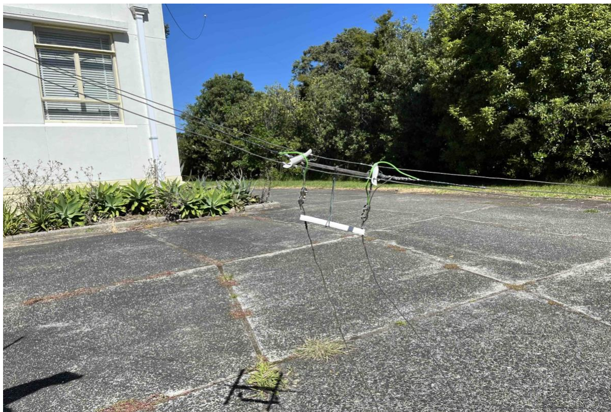
The (again) repaired dipole-no solder burns this time Dave! Dave provided the stainless steel clamps- which should last for at least another 40 years-even if the copper wire doesn't.
