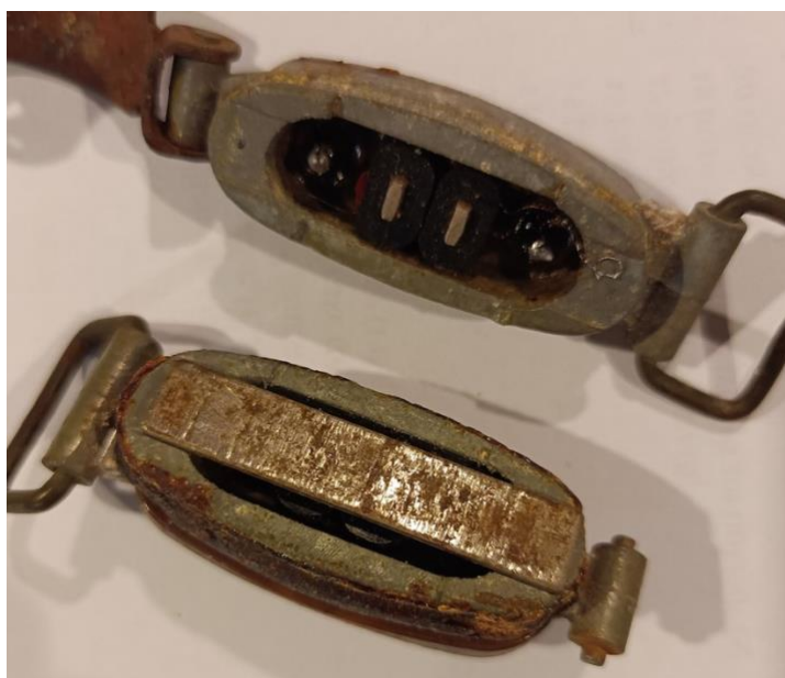
What is inside a (rusty) WS38 Throat Microphone.
