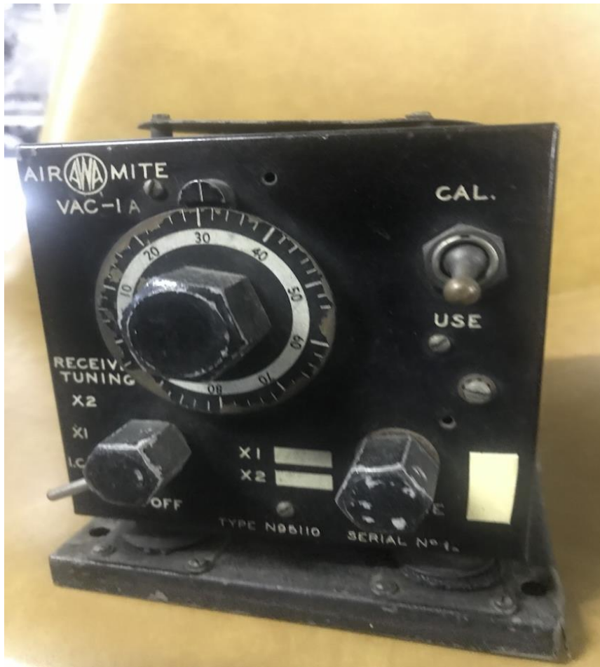
Early Aircraft radio receiver from Tiger Moth made by AWA.
