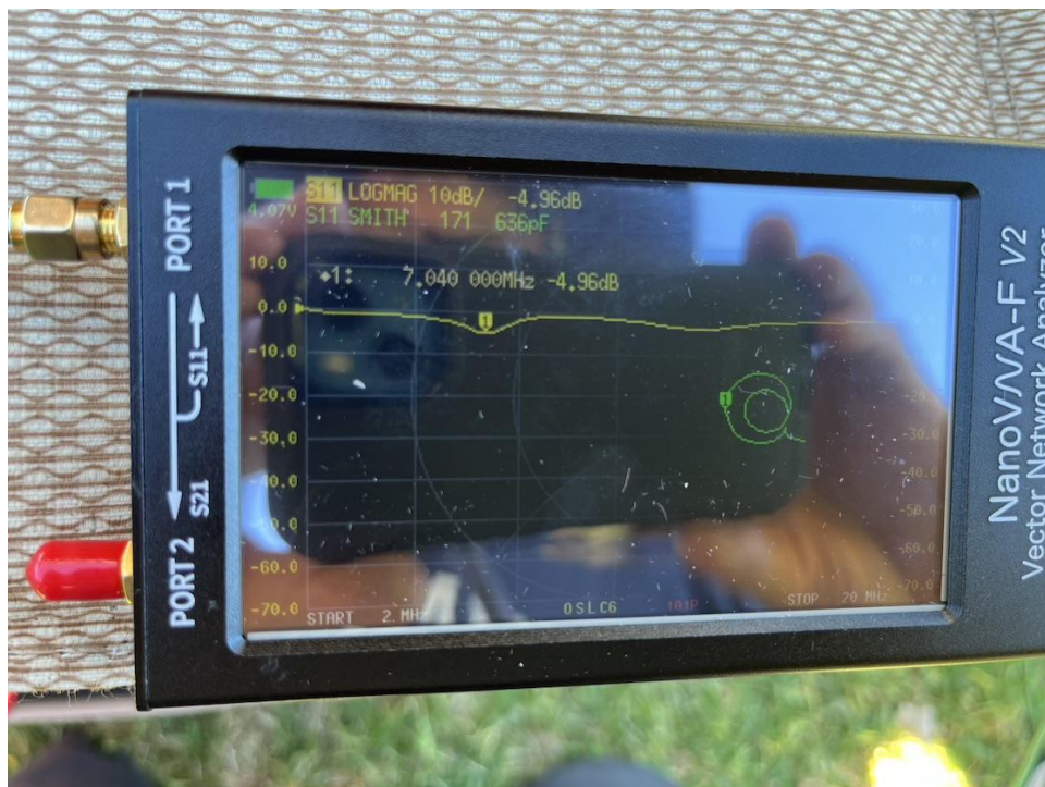
VNA connected to series capacitor and earth using crocodile clips.
