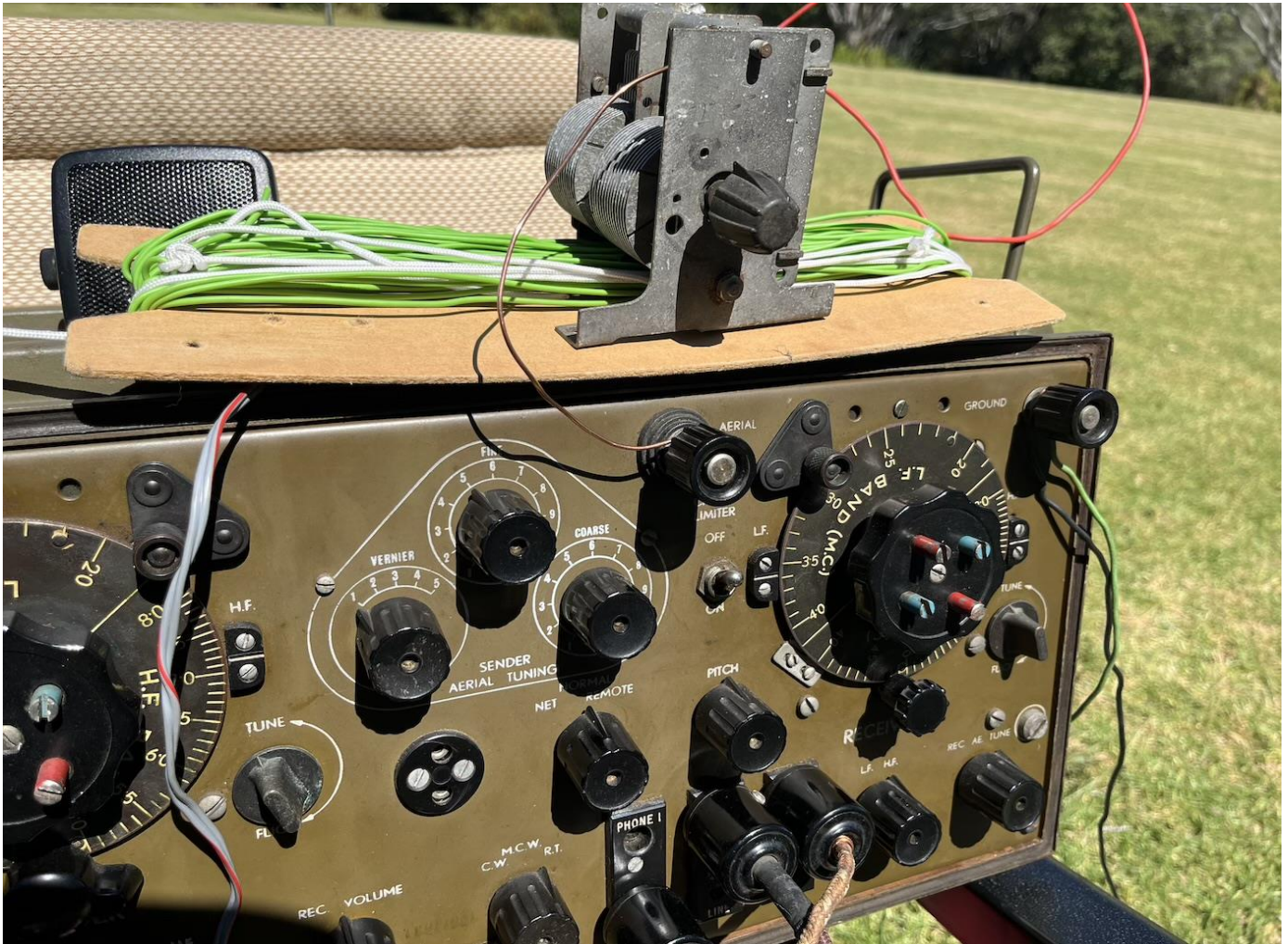
ZC1 with variable cap and earth wire. (The rolled up wire is being used only to insulate the capacitor from the set)
