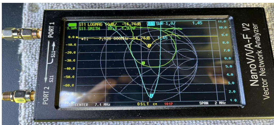
VNA of the "Pack 12" portable aerial set for 40 meters. Nice resonant point at 7.120 MHz
