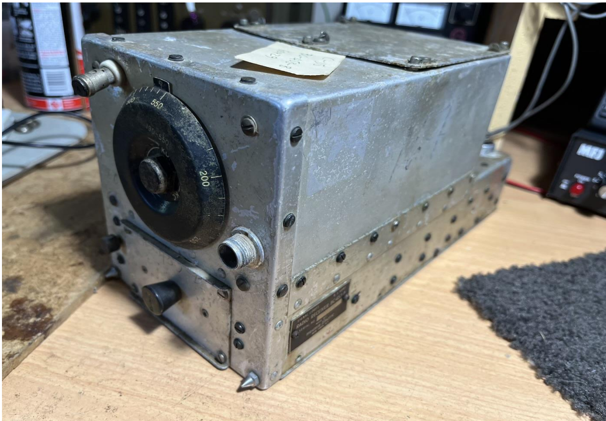
An original unrestored Aircraft Radio Corporation (ARC) Beacon receiver, obtained from Dr. Brian Clarke, Sydney, Australia. Model is a BC-453-B, 180-550KHz. The small plate below the dial would normally be replaced by a special connection box for the NDB compass mounted in the pilot's instrument panel. Tuning is by Bowden cable to the pilot's radio control head.
