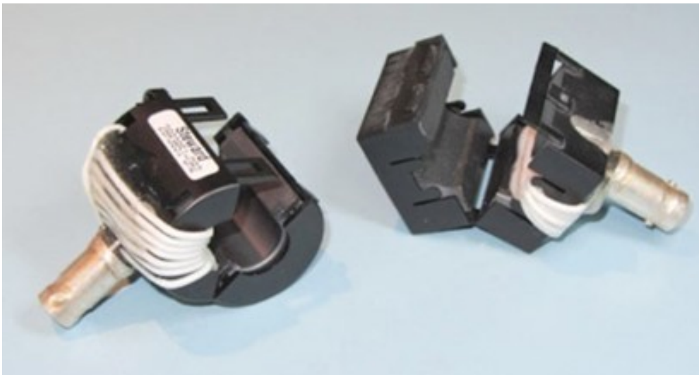
Figure 3. An example of simple current probes you can make to measure harmonic RF currents in cables.
