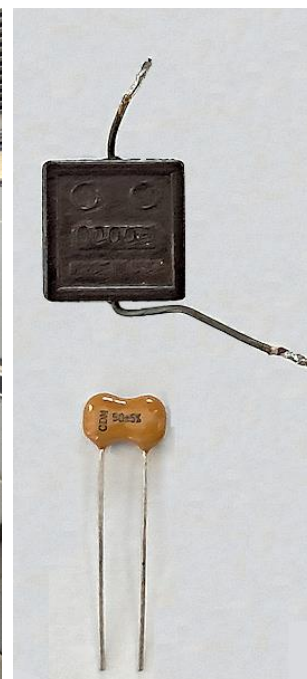
Out with the old and in with the new – 50pF Silver Mica caps
