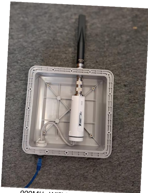
900MHz WiFi Ready for Testing
