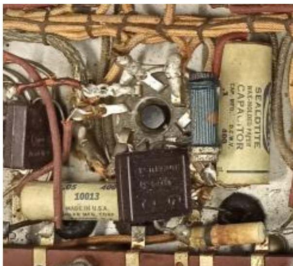
Solar capacitors in the mixer stage of 941SWB
