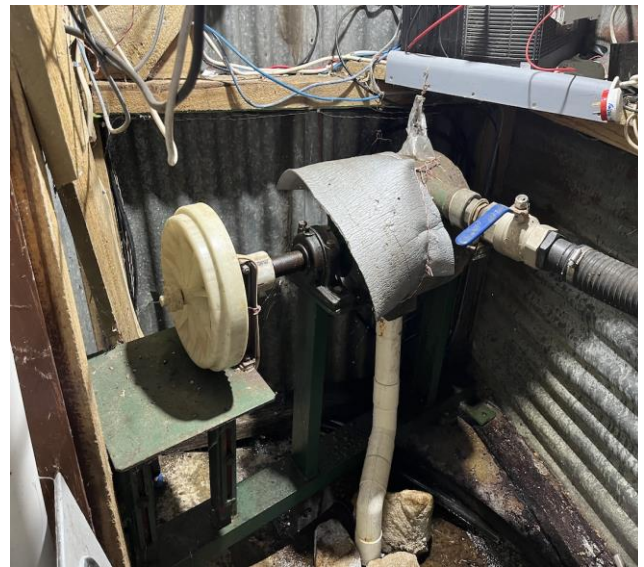
Alternative power source- a repurposed "Gentle Annie" motor
