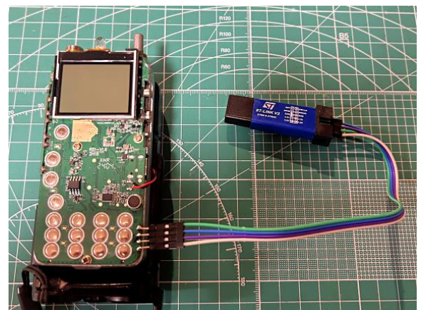
ST-Link Programmer Attached
