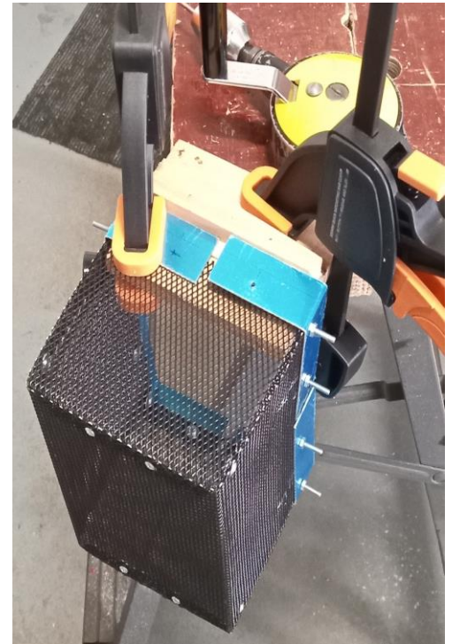
Riveting the safety cover
