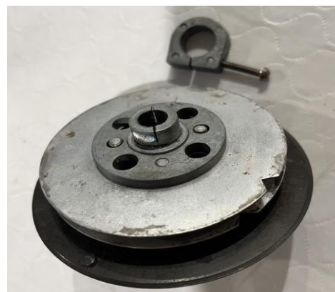
Dial removed, showing the tuning capacitor clamp with set screw and the groove where it fits on the dial hub.
