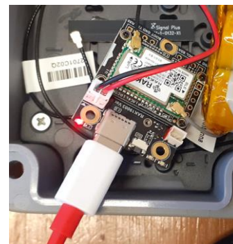
The Meshcore Radio – not much bigger than the USB cable being used to program it !
