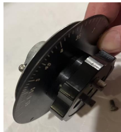
New dial plate installed on hub, centre set screw shown
