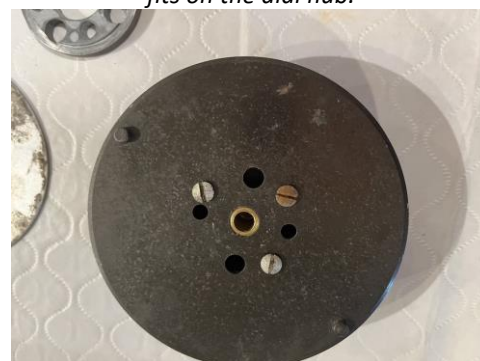
Back side of knob/plate assembly, showing the three 'offset' dial plate attachment screws.
