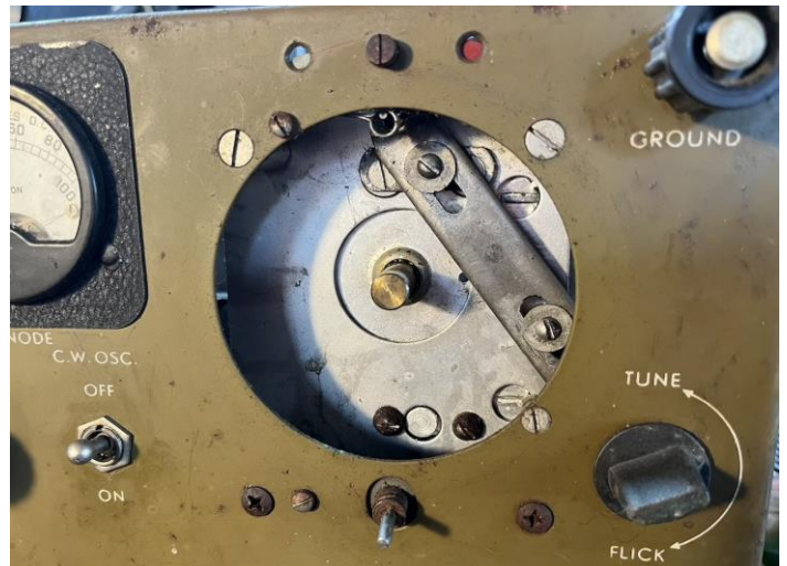
This is the Mk.1 set with the receiver dial mechanism and fine tune pulley removed
