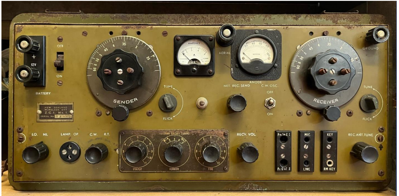
Finished! ZC1 Mk1, Version 1 (with RF ammeter) now with replaced frequency dials. – now about the other corrosion....
